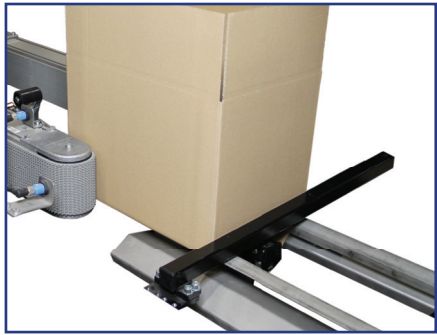
Square Case Transition A pusher bar, parallel to the rear wall of the case, pushes it into the sealing section where spring-loaded side belts automatically adjust for any width variations.
